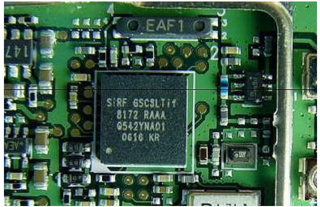
Figure E-2. 2010 CPEX Evaluation of Automation in Field Data Collection in AC: GPS Chip
